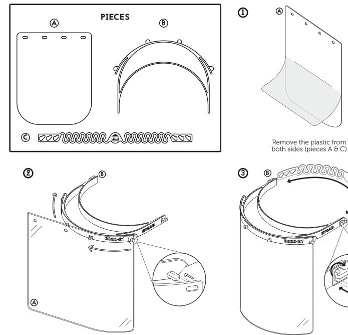
Mount the protection over the visor, inserting the holes in the 4 pivots, starting on one end. The last pivot comes under preassure. Attach the strap to the back. The piece has with multiple grooves to adjust the distance.
